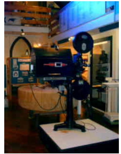
Working film projector on display in the Museum—as was used in the Devonport Picture Theatre
